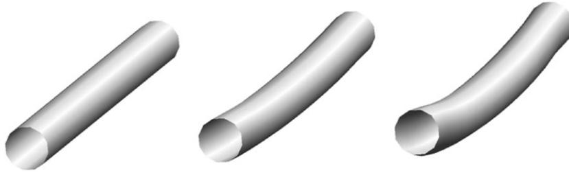
Figure 24. The bending deformation in a (10,0) tube resolved from the multiscale concurrent model.
