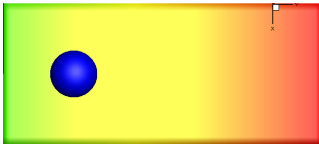
Fig. 6. 3D Computational model of cell spreading on a stiffness-varying substrate, the color in the substrate stands for different stiffness, the stiffness at the right end is the highest (top view). (For interpretation of the references to color in this figure legend, the reader is referred to the web version of this article.)
